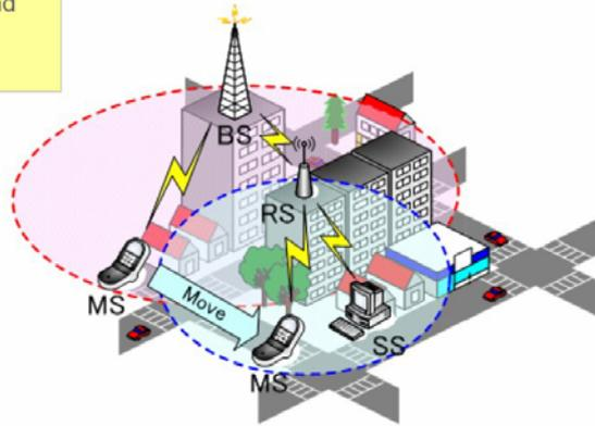
Figure 28 802.16j multihop relaying (a subset of mesh) [Nortel]
