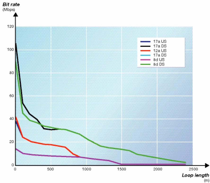
**Figure 12 VDSL bandwidth versus distance (for various crosstalk conditions) [Ericsson 2006]**
