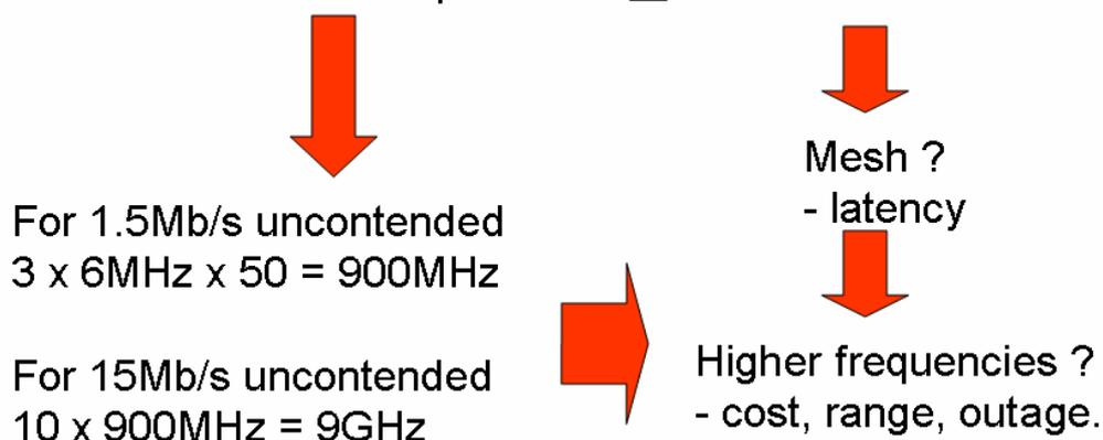
Figure 50 Eliminating 50:1 contention - ADSL versus 802.22 wireless examples
