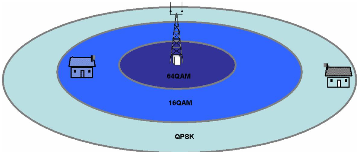
Figure 48 Modulation format versus location in cell
