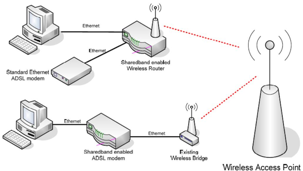
**Figure 58 SharedBand using wireless access**
