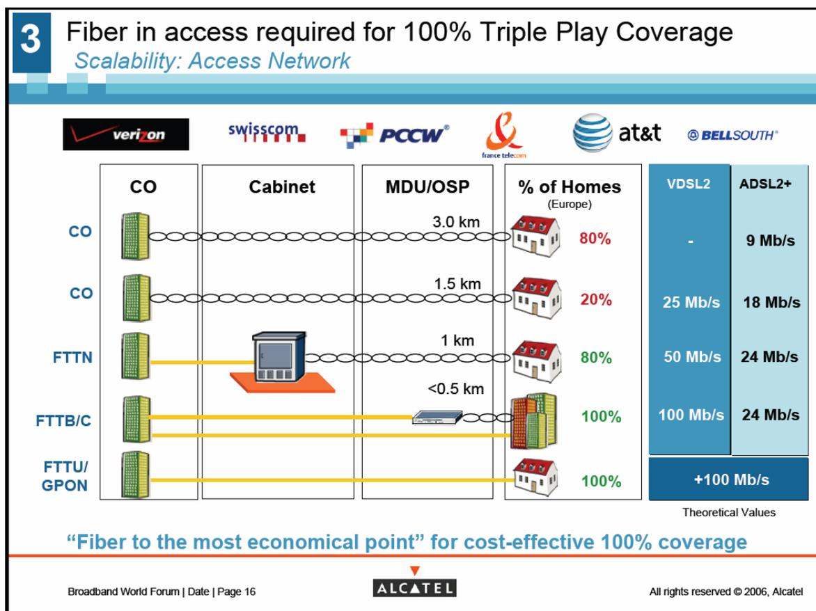
Figure 51 Fibre to the x, where x is the most economical point [Alcatel 2006]
