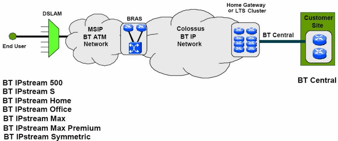
Figure 23 BT's own diagram of the IPStream architecture [source: BT SIN 386]
