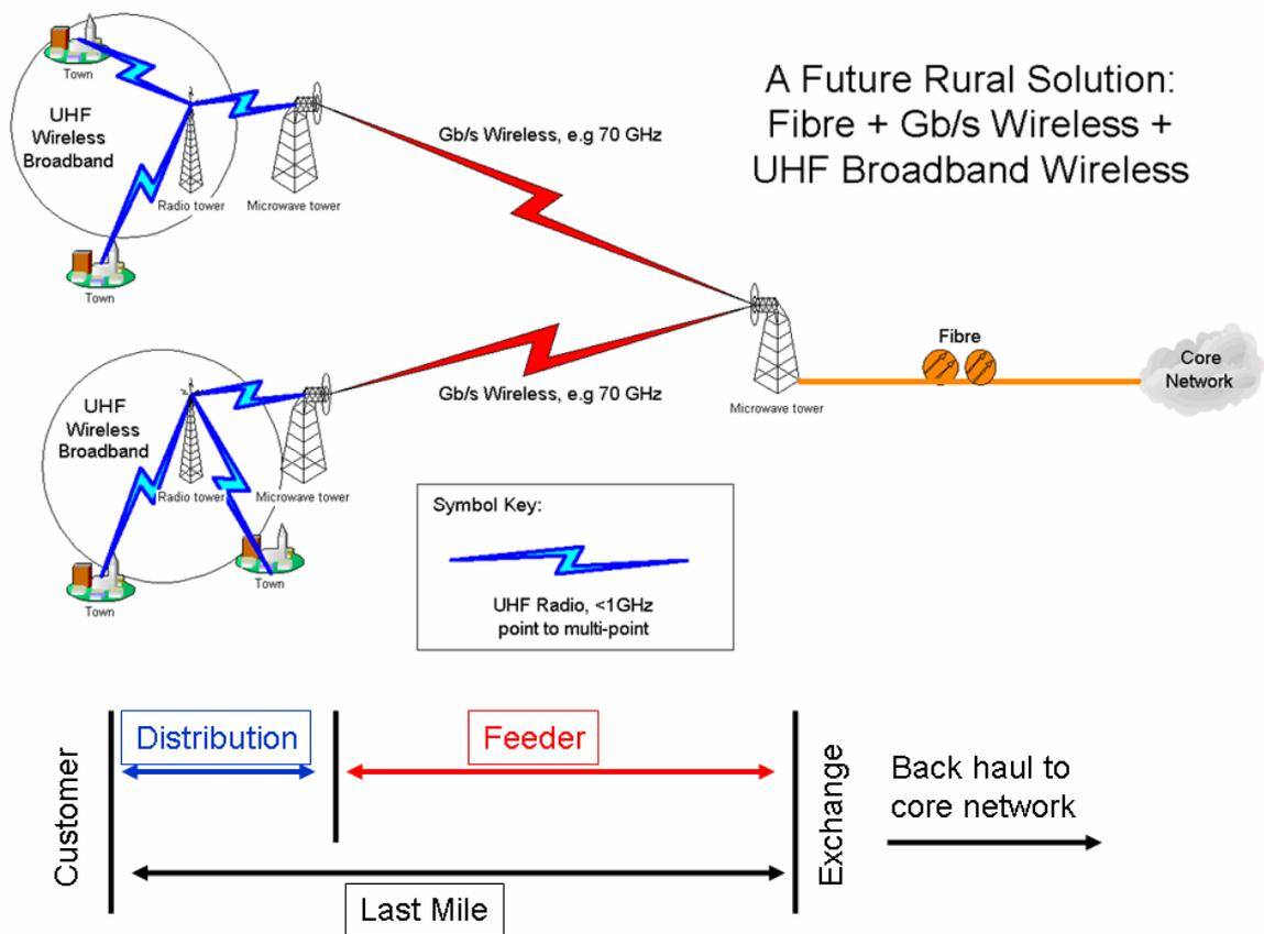
**Figure 31 Last mile distribution (UHF), feeder (Gb/s wireless) and back haul (fibre) segments of the network (repeated figure)**
