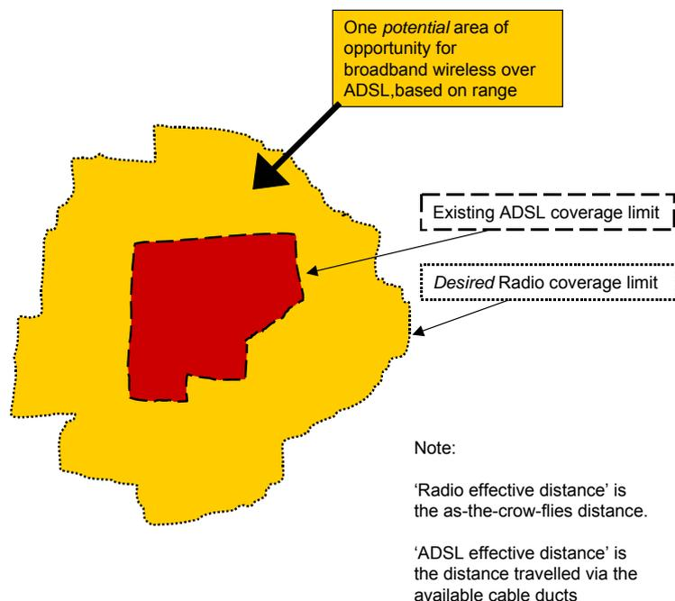
**Figure 22 Radio versus ADSL coverage contours**
