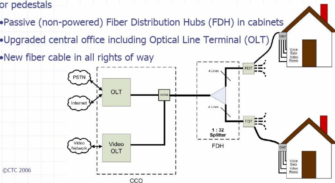
Figure 36 Verizon's FTTP architecture, according to CTC
