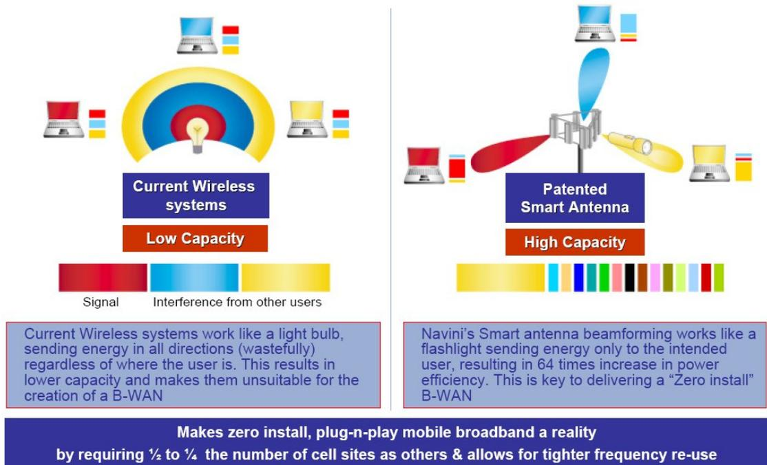
Figure 20 Beam steering is essential for economic WiMAX indoor/mobile operation [www.navini.com]
