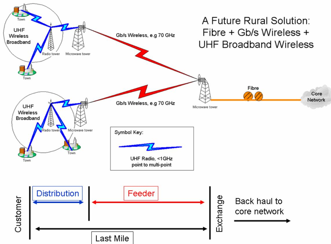
Figure 4 Last mile distribution (UHF), feeder (Gb/s wireless) and back haul (fibre) segments of the network
