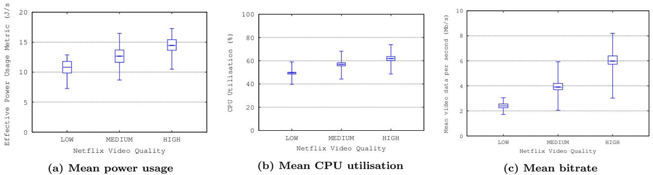
**Figure 2: Summary of the resource usage (energy, CPU and network) for playback of the entire corpus of Netflix videos at the available quality levels. The corpus consisted of 202 videos. Each data point is the mean of 5 runs, each of 120 seconds in duration.**
