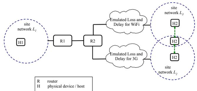
**Figure 3: The topology for the experiment.** The hosts H1 and H2 reside in different networks, with Locator values of  $L_1$  and  $L_2$ , respectively. The green / dashed arrows identify movements of H2 between site networks generating a handoff.
