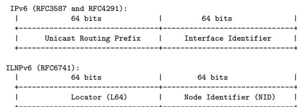
**Figure 1: Encoding of NID and L64 values into the IPv6 address bits. An ILNPv6 L64 value has the same syntax and semantics as an IPv6 routing prefix. An ILNPv6 NID value has the same *syntax* as an IPv6 Interface Identifier, but different *semantics* as it represents the *node* not an *interface*.**
