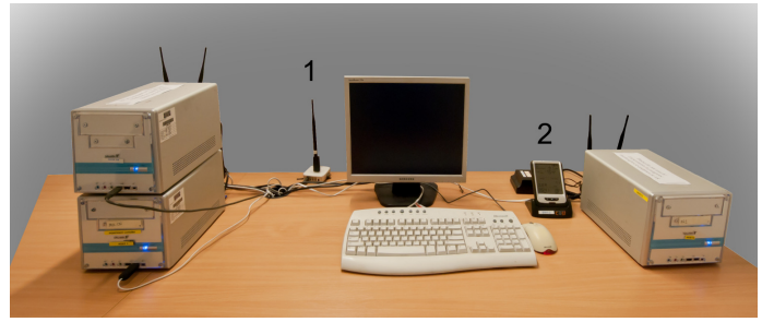
Fig. 3. Some nodes from our testbed. 1. The WiSpy DBx probe with antenna, mounted in a desktop USB hub. 2. The CC128 power meter and its power clamp (behind the CC128 LCD screen).
