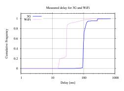
Figure 4: The cumulative frequency distribution of one-way delay of WiFi network and 3G network.
