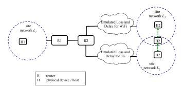
Figure 3: The topology for the experiment. The hosts H1 and H2 reside in different networks, with Locator values of  $L_1$  and  $L_2$ , respectively. The green / dashed arrows identify movements of H2 between site networks generating a handoff.
